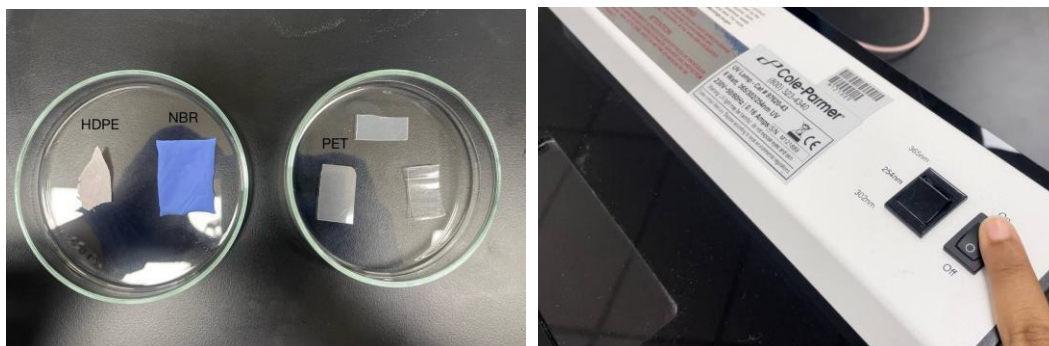
Fig. 1 Samples before UV exposure using a Cole Parmer UV lamp
