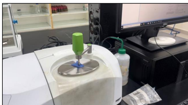
Fig. 2 The polymers were analysed using Spectrum two, Perkin-Elmer, USA
