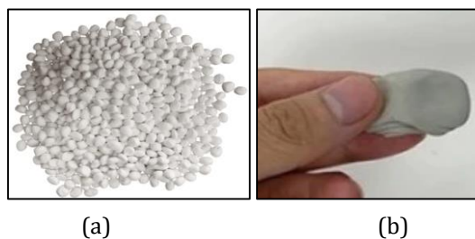
Fig. 1 (a) Plastic pellets as the “Masterbatch Pellets”; (b) Putty filler used (5 - 6 mm in size)
